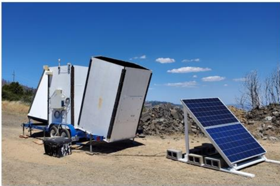
Figure 4. Photograph of the ACS Model 2000 Sodar at the upper-air monitoring site near Cobb Mountain, California.
